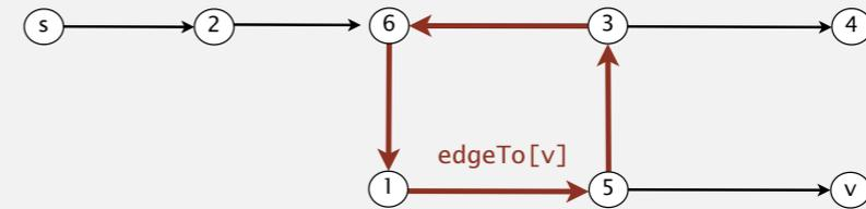
**Proposition.** If any vertex `v` is updated in pass `v`, there exists a negative cycle (and can trace back `edgeTo[v]` entries to find it).
